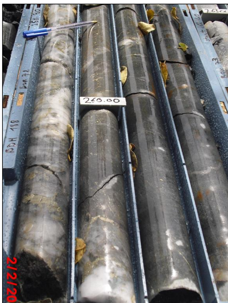
Figure 10: Drill core from hole BDH188, Netiana Lodes, Balogo Project, 258.5 m to 262.4 m, showing thick quartz vein and possible high-grade mineralisation Source: D. Williams, 2017
