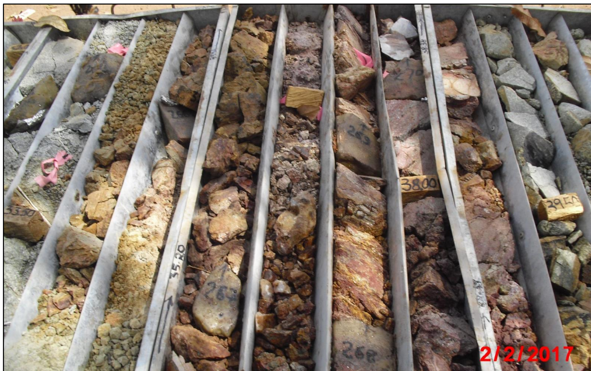
Figure 22: Drill hole BDH046 (Netiana Lode, Balogo Project) showing weathering profile and billets chosen for BD measurement.
