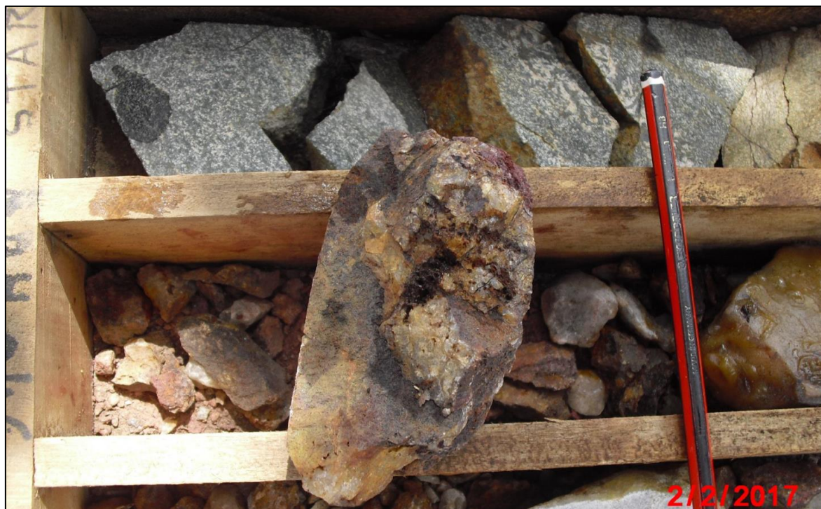
Figure 23: Drill hole BDH046 (Netiana Lode, Balogo Project) very high grade Au (>500 g/t) 43.5 m - 44.2 m
