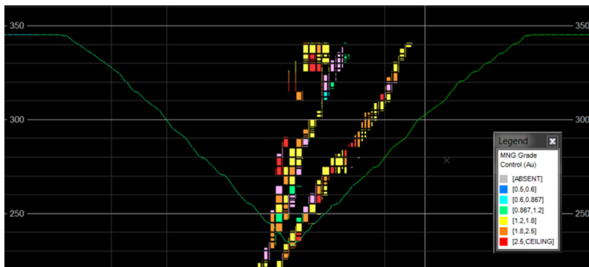
Figure 56: Section A-A showing Mineralised Blocks (> 0.7 g/t Au) and the Pit Limit
